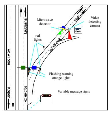
Figure 2: Layout of the wrong way detection system in the area of exit ramp H5 for Trieste
