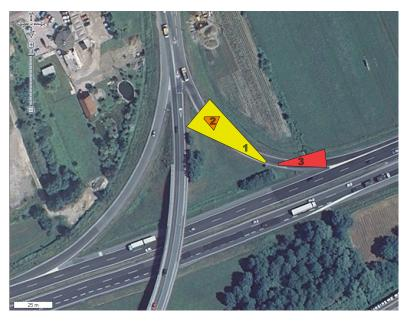
**Figure 6:** Example of system layout with three radar detectors
