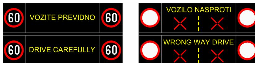
**Figure 4:** VMS signs in a case of wrong way incident; unconfirmed alarm (left), confirmed alarm (right)
