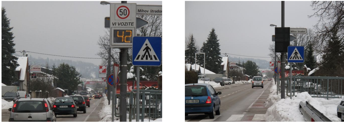
Figure 2: View of the radar speed display visible (left) and display hidden (right)
