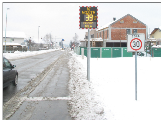
Figure 4: View of the radar speed display and speed limit sign on Brezovica site
